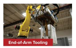
Multiple pre-engineered, in-stock EOAT units are available including our popular clamping tool with pneumatically-powered support lip.
