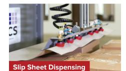
Quick-Ship Palletizers can be designed with a slip sheet hopper and standard EOAT that automates the placement of anti-slip sheets on each pallet.
