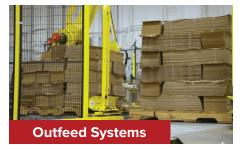
Pre-engineered pallet stations can designed for manually operation or feature integrated discharge conveyors for a higher level of automation.
