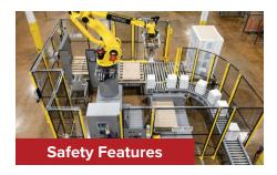
All cells are designed and configured with the appropriate safety fencing, light curtains and other systems to comply with category 3 safety standards.
